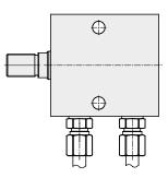
Manifold mounting versions with O-ring sealing
